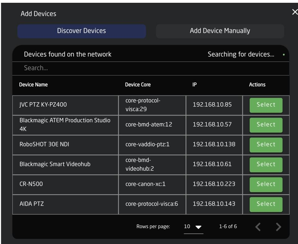
Pressing SHIFT + the green Select button will allow for multiple device selection.
