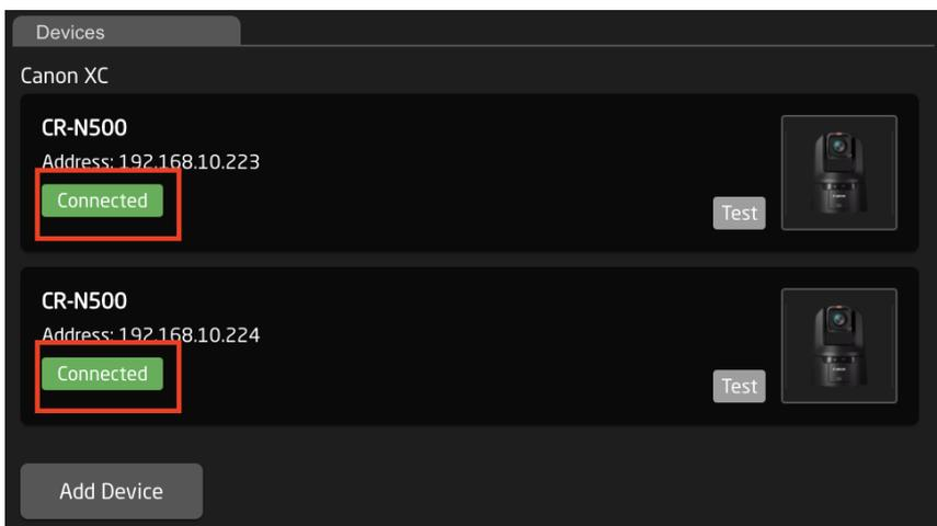
Clicking on a device name in the Devices section will open up the details. Here the name, ID number, and Active status of the devices can be changed. By default the controller name will be
