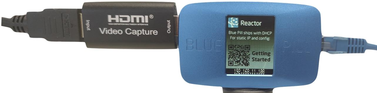
Please note, some PTZ camera models natively support thumbnail presets like the Canon CR-N500. The FrameLink package, Framelink Window, and the HDMI Video Capture stick are not needed for those models of cameras. This is only for cameras or other devices that do not natively support this feature.
