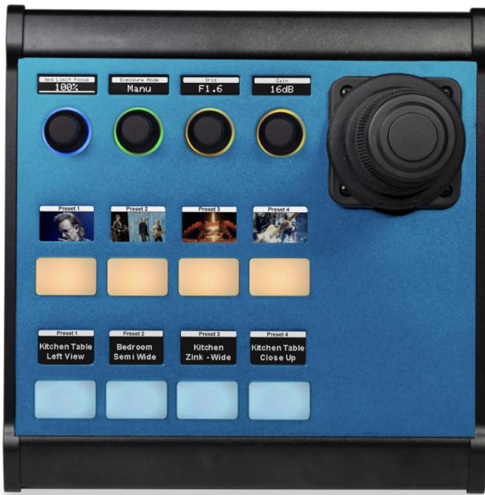
The Skaarhoj Frame Link package combined with an HDMI Video Capture card allows for thumbnail preset images on compatible SKAARHOJ panels like the MKA1, MKA2, and future color display controllers from any HDMI source.
