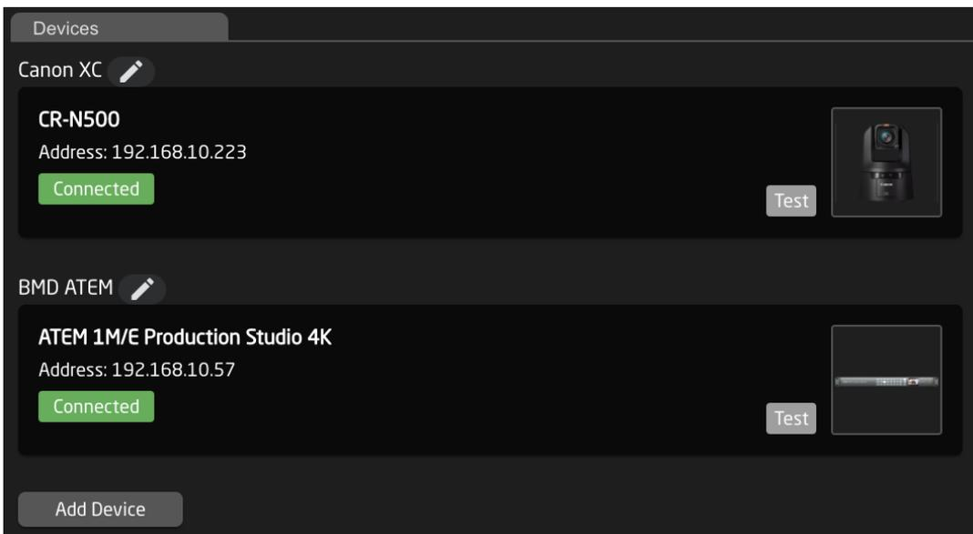
Clicking on a device's name in the Devices section will open up the details. Here the active status, IP address, Username and Password, Device Name, DeviceID, ModelID, and Description can be adjusted. (Details shown here are for a Canon CR-N500 PTZ camera, available detail options are device specific) . The device name and description are customizable. The device
