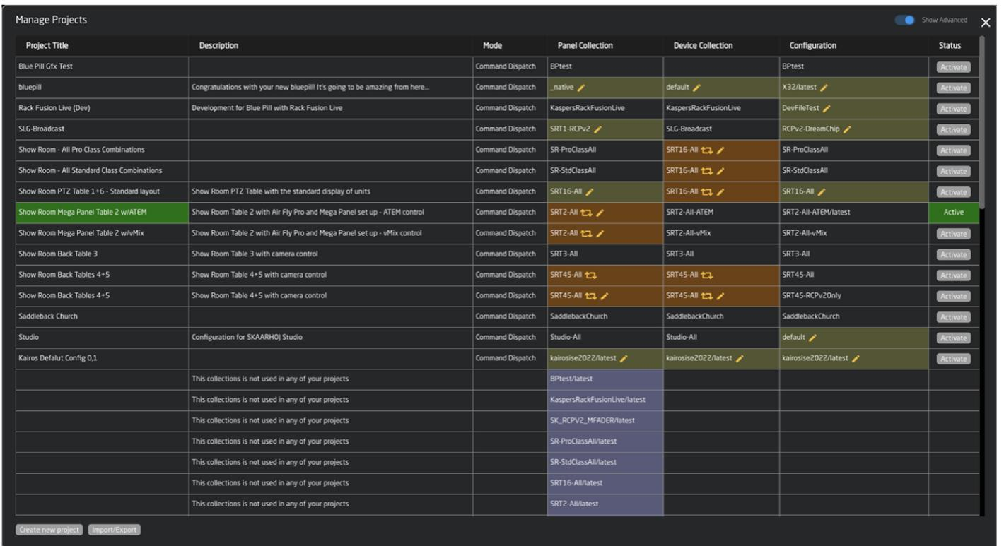
Unlike UniSketch where a change of configuration and device cores needed an online connection to SKAARHOJ server, on Blue Pill everything is stored locally in Reactor. Only software upgrades or installations of non-existing device cores and applications need communication with the server.
