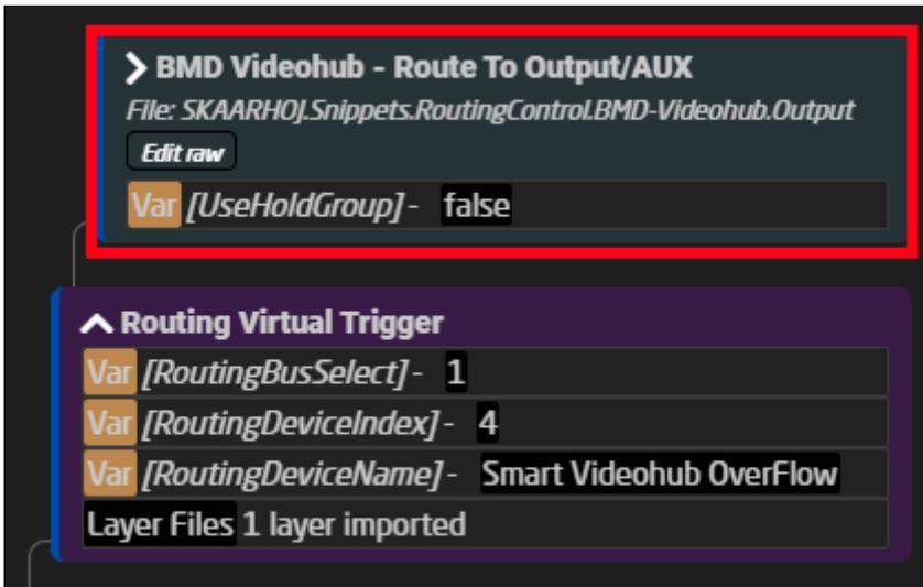
Inside it has virtual triggers that read the stored routing flag and sends the routing selected and sends it to the parameter on the Videohub.
