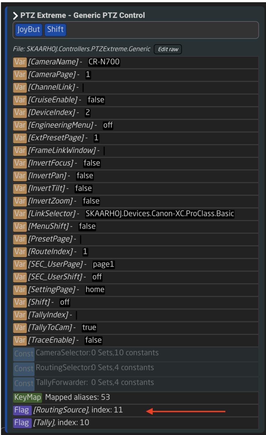
When managing multiple PTZ Extremes with the same configuration, a conflict arises as each controller's Routing Trigger setup uses the same index (11). This duplication can lead to operational issues. That same is true for other controllers and their configurations being shared.
