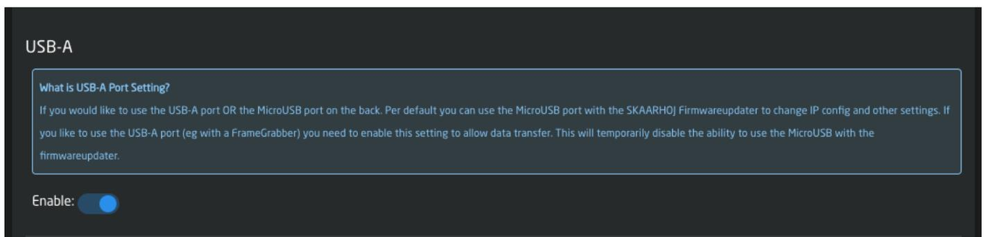
2. Plug in a USB to Ethernet Adapter into the devices USBA port and wait about 5 seconds, then refrehs the settings page in your browser. You should now see an "Other" tab in your network settings, that will let you configure the IP settings for the external connection.
