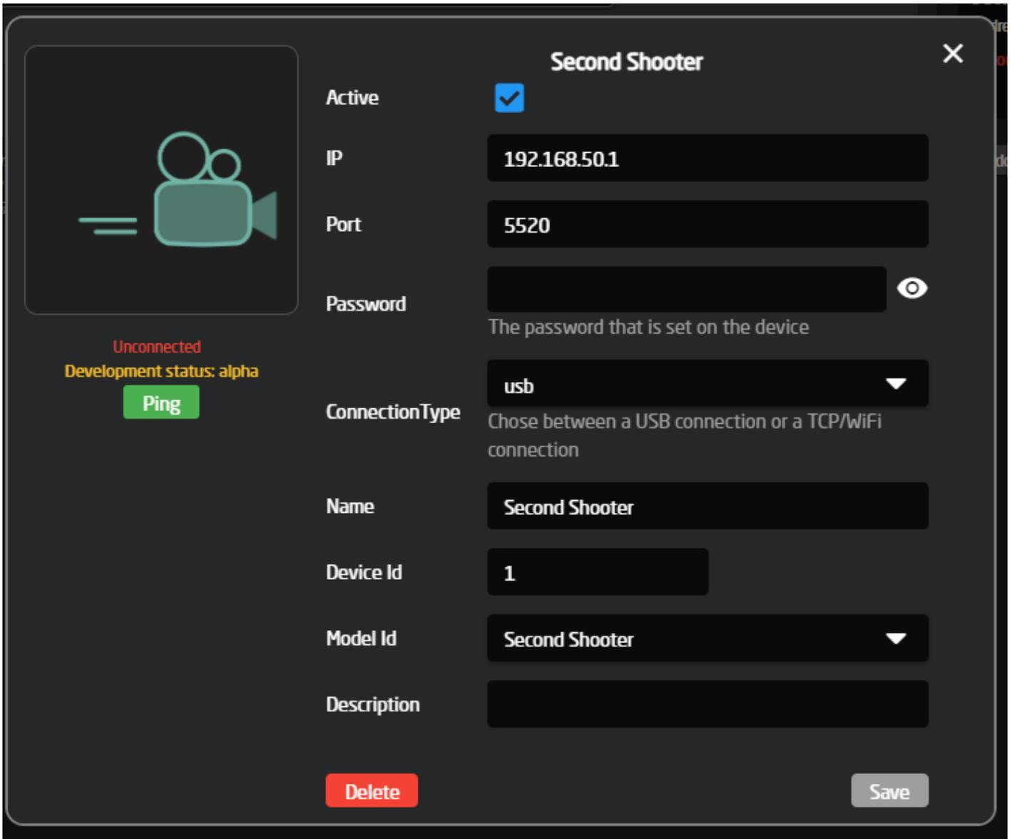
If your config box does not have the "Connection Type" option, please click the save button and wait until you see the device on the left side say "Disconnected" or "Connected". If it's your first time installing the core, it will say "Installing Core" wait for that to finish, then restart reactor to load the new Device Config structure.
